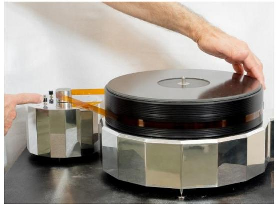
**Step 7:** Set/check the starting belt tension.
